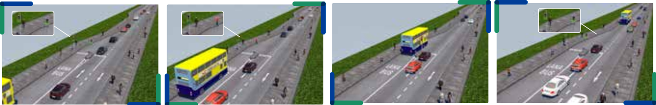
1. Traffic proceeds as normal. 2. As the bus approaches, the light signal changes to halt general traffic. 3. The bus has priority to proceed. 4. When the bus has cleared the junction, general traffic proceeds.
